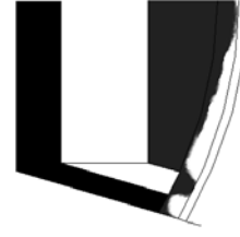
Fig. 1. Optimal shape of the rotor iron part.
